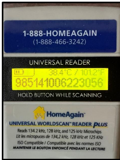
The Bio-Therm chip displays both the horse's ID number and body temperature when scanned
